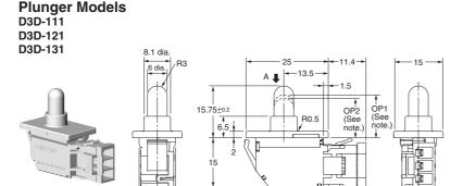
Note: The dimensions OP1 and OP2 apply to the D3D-111 only. The D3D-121 and D3D-131 are SPST-NC and SPST-NO respectively and so therefore have only one corresponding dimension here (OP).
